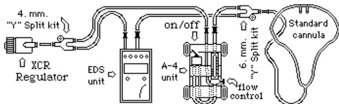
This figure (below) shows the most popular back-up bypass arrangement for the dual EDS systems. The second set of "Y" split kit connecting the EDS units and the F-2 mask kits are the self-sealing type. The auxiliary opening will stay sealed until the 4 mm. inlet tubing of the F-2 mask kit is plugged in for emergency service.
