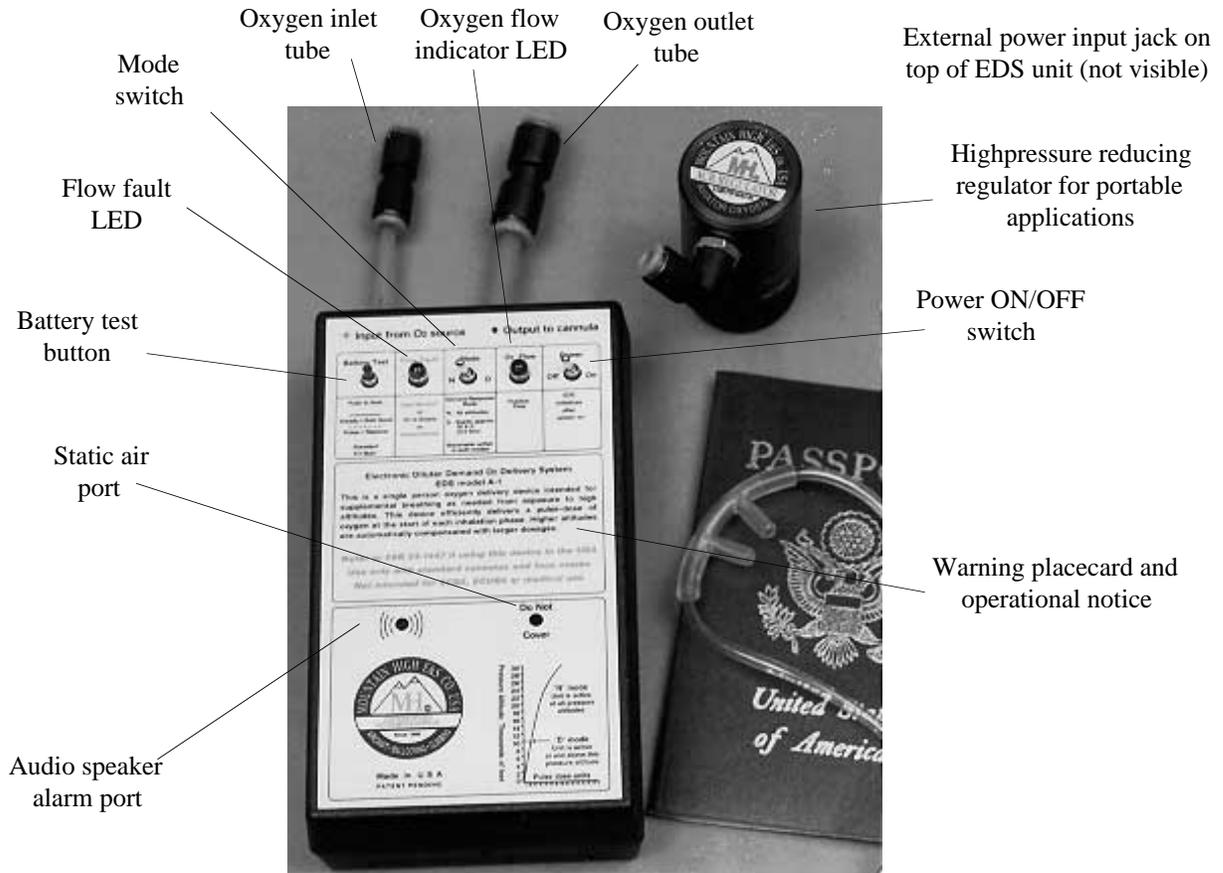
The battery test button places a load on the battery in order to detect battery failures within the next few hours. Oxygen will flow during depression of the battery test button. The battery test button energizes the oxygen admission valve by bypassing the electronic circuits of the EDS unit serving as an emergency supply of oxygen.
