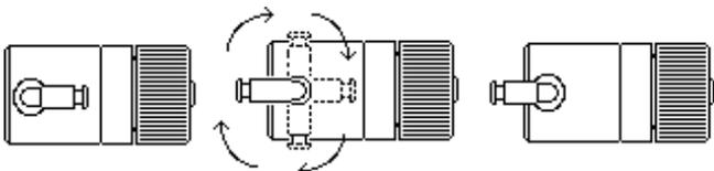
The quick-connector rotates to any direction desired
