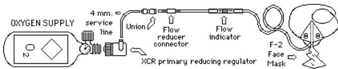
The second most common method uses a self-sealing "Y" with the F-2 mask where the pilot would simply connect the 4 mm. inlet tube of the F-2 to the "Y" for emergency service. This provides the best and easiest to use back-up system for single pilot applications. In addition, an option for adding a delivery device for a future passenger is provided.
