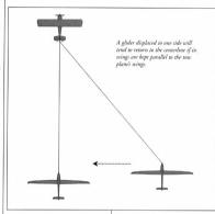
"sweet spot" and keep it there. By doing this we will descend and gradually round out into the proper position. The same is true for climbing back from a low position. Students should learn that when the tow plane is not viewed in the "sweet spot" we will soon drift out of position.
