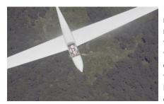
~500 feet lateral separation. As I approach, I reduce power and lower full flaps to reduce overtaking airspeed. However, rarely can I match the glider speed. As the Pawnee pulls AHEAD of glider, and the glider
