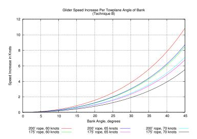
Figure 5: Technique B Glider Speed Increase
