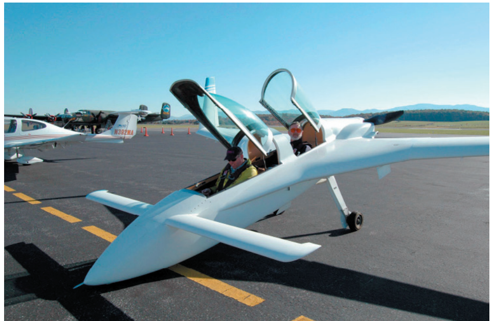
Joe Parrish (front) and Jim Kellett preflight Joe's latest commuter vehicle, a canard wing, pusher aircraft called a Berkut, before a tour over the Virginia countryside, Oct. 26.
