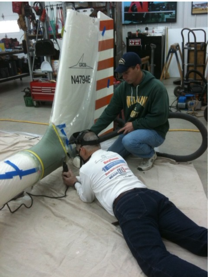
A dolly was started by making the fiberglass boot. The wheel still needs to be mounted and the boot finished but we have a dolly!
