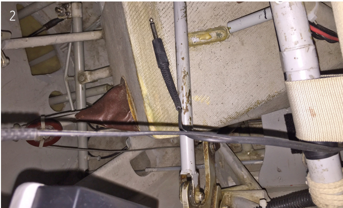
2-Here it is shown on the fiberglass box aft of the seat. The aileron crank is seen at the bottom of the picture.
