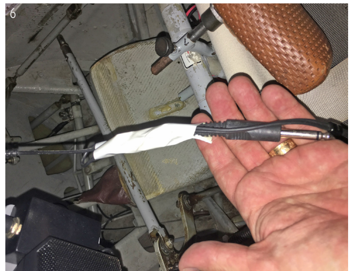
6-As a temporary measure, the plug has been taped to the cable to keep it restrained.
