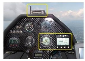
gets within a few miles and reads out the altitude difference, it is often my first warning that there is somebody nearby. The Cambridge 302/303 takes a 12v power supply, pitot and static inputs, uses included GPS to figure winds and navigation data with final glide and speed to fly, also has a wiring harness to connect to an Oudie. Both work fine and have served well, let me know if you are interested in either.
