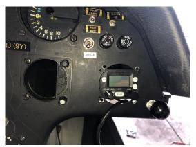
his hangar. The ADS-B OUT transponder and other equipment was purchased for \$3,421.29. The equipment has been installed, but the system is displaying a fault. On Wing in Winchester is working with TRIG on the troubleshooting of the transponder.
