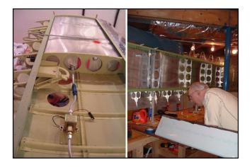
Left: Outboard wing with top aluminum skins off and shows the extra fuel tank with transfer pump. The outboard fuel can be pumped to the inboard main fuel tank (not shown). A bell crank is shown for the ailerons. Right: Father-in-law shown with a wing mounted in a jig to ensure it is square – no twist.
