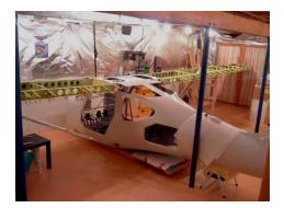
Setting the dihedral angle in the basement. It is set with a little trigonometry, and a 35foot string (barely visible) and bubble level; it is low tech but effective.
